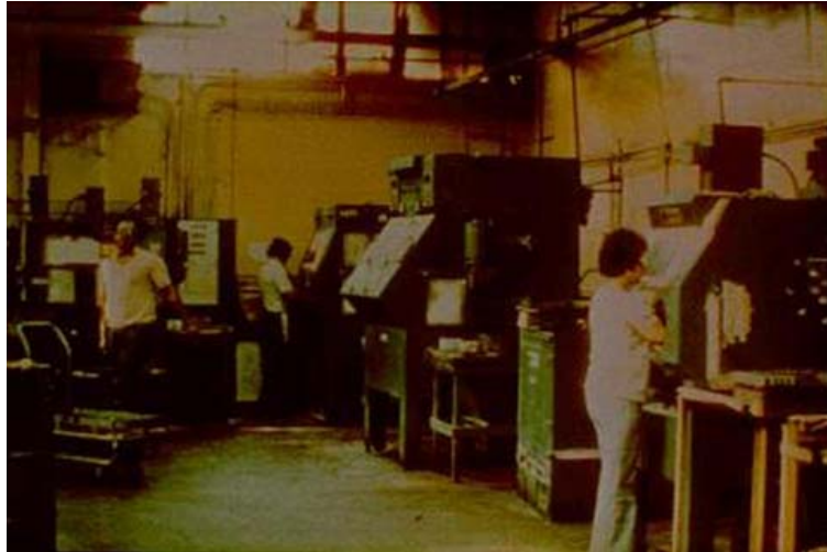
Figure 43. Workers performing operations with local exhaust systems installed
